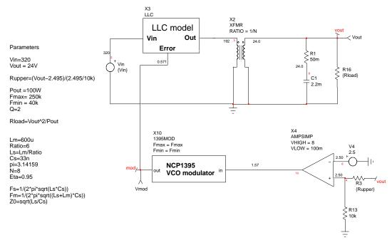
Figure 16. The complete test circuit including the LLC DC model and its VCO modulator.
