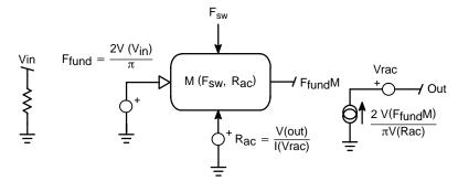
Figure 8. The model looks for the current circulating inside  $R_{ac}$  and forces a proportional current on the output node.
