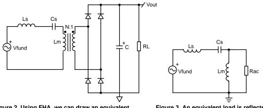
Figure 2. Using FHA, we can draw an equivalent "sinusoidal" schematic of our LLC converter.
