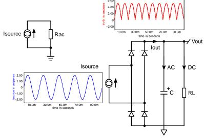
Figure 4. A simplified representation helps us to derive  $R_{ac}$  in a few lines of algebra.
