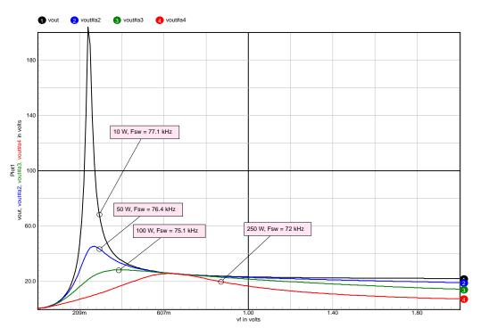
Figure 19. Frequency Evaluation for Variable Load Conditions, Input Voltage is 350 Vdc
